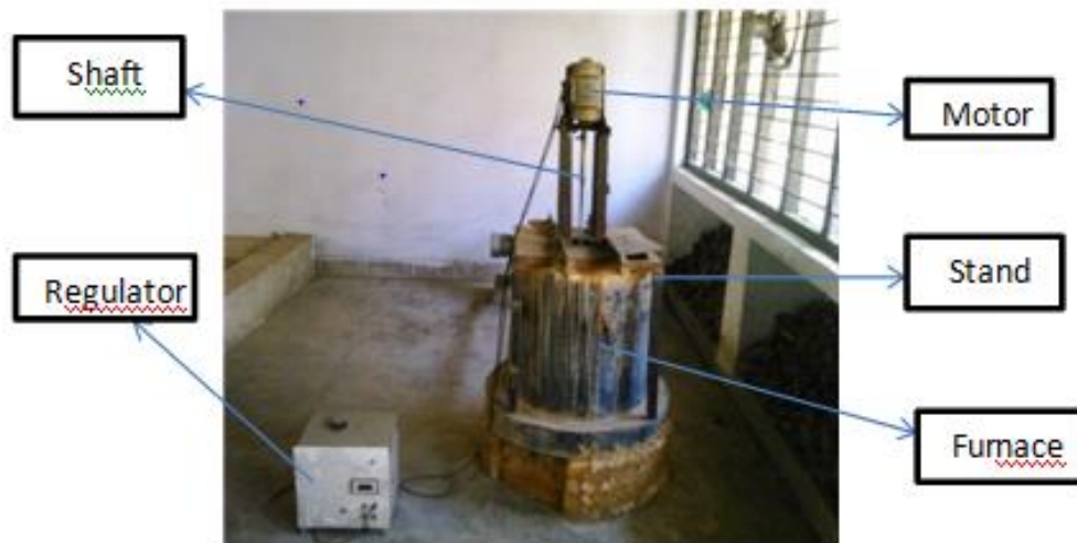
Fig.1. Assembled Setup for foam manufacturing
